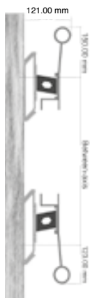
The projection surface is tensioned with eyelets at the back of the frame.
