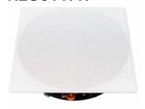
Square speaker for either in-wall or in-ceiling mount, 5,25" coaxial driver 0.75" titanium dome tweeter tiltinge and built-in 100V / 70V transformer box. 120° wide coverage. ABS chassis and stainless steel round protection grille painted in white or black.
