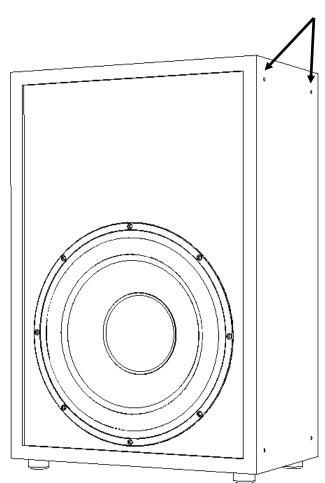
Standard Inserts Mounted on All 4 Faces for Installation Flexibility
