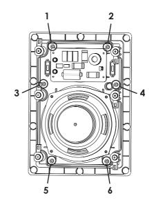
**2 - Opening the fixing brackets**Rotate the 6 fixing brackets outwards.
