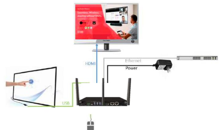
myTeamSharer transmits image and audio signals as well as touch input to a display at the same time. myTeamSharer supports the USB-HID protocol. For example, interactive touch displays, projectors or whiteboards as well as a mouse can be connected to the base via USB in order to:
