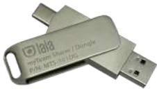
**MTS-102DG:** Full function USB-C with Display Port Alternate Mode interface, which supports Audio and Video transmission. This PC's type C connector also requires full function type C connector for mirroring screen.
