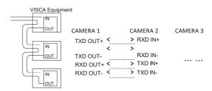
Using RS232 cascade connection almost the same as RS422. The output of camera #1 connect to the input of camera #2 and the output of camera #2 connect to the input of camera #3 and so on:
