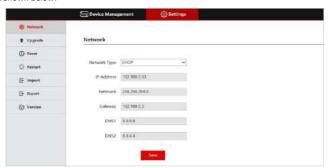
Dynamic Address(DHCP)(Default acquisition method):The joystick controller will request an IP address from the router automatically. After the request is successful, it will be displayed on the joystick controller's display. The display format is: "Local IP: 192 168 x xxx"
