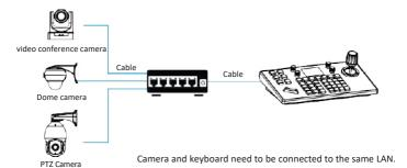
Connect the camera and joystick controller in the same LAN and ensure their IP address in the same network segment. Such as 192.168.1.123 & 192.168.1.111 belong to the same network segment, while 192.168.1.123 & 192.168.0.125 do not belong to the same network segment, then you need to modify the joystick controller or the ptz camera ip address at this time. The joystick controller get its IP address
