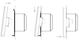
3. Carefully tighten the fixing screw to fix touch panel on the wall
