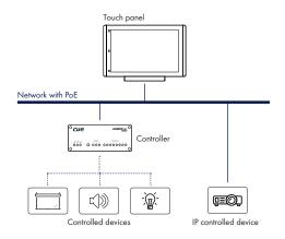
The following diagram describes the use of touch panel with IP controlled devices only. This configuration allows to create cost effective distributed control solution where touch panel serves as controller and graphic user interface in one box. In Cue Visual Composer touch panels and controllers are programmed in the same way, which makes possible to use touch panels as fully functional control units.
