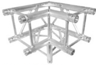
3-Way 90° Corner CT290-4390C • Size: 11.42 x 11.42 in (290 x 290 mm) • Weight: 16.53 lb (7.5 kg)
