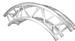
2.0 m arc section CT290-420CIR-90 • Outside diameter: 6.56 ft (2 m) • Inside diameter: 4.92 ft (1.5 m) • Arc: 90° • Weight: 21.6 lb (9.8 kg)
