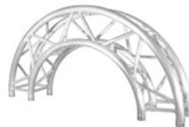
1.5 m arc section CT290-415CIR-180 • Outside diameter: 4.92 ft (1.5 m) • Inside diameter: 3.28 ft (1 m) • Arc: 180° • Weight: 21.6 lb (9.8 kg)
